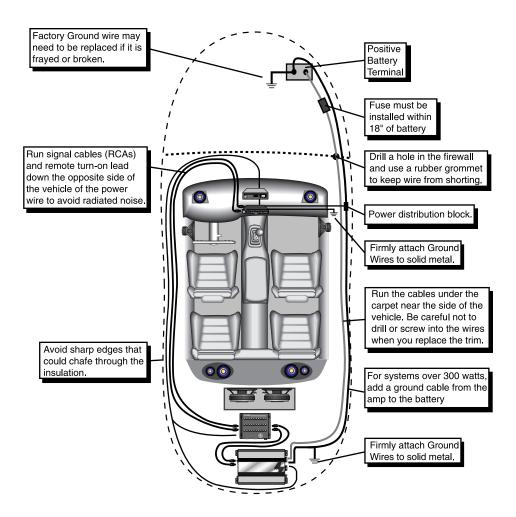
Before beginning, disconnect the negative (-) terminal of the battery prior to working on the positive (+) terminal to prevent a short to ground. This is important, unless you want to spend the rest of your life with a nickname like "Sparky," or "Smokey." Reconnect the negative terminal only after all connections have been made.
