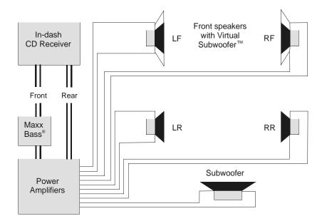
**WARNING:** If you are using a source unit with bridged high powered (or "floating ground") speaker outputs, a suitable high to low level adapter must be used. If you are unsure about your head unit see your local *PrecisionPower*<sup>m</sup> dealer.
