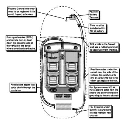
Warning! A Main Fuse must be installed within 18" of battery!
