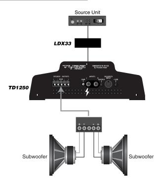
(Two four ohm subwoofers connected in parallel = two ohm load on the amplifier.)
