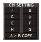
& 3 / A & C) are matched, as right channels (2 & 4 / B & D). Crossover settings remain independent. Channels 5 & 6 (E & F) are independently variable for equalization and crossover settings, as are channels 7 & 8 (G & H) for subwoofers. This configuration is ideal for advanced 3-way component applications using all active crossovers.
