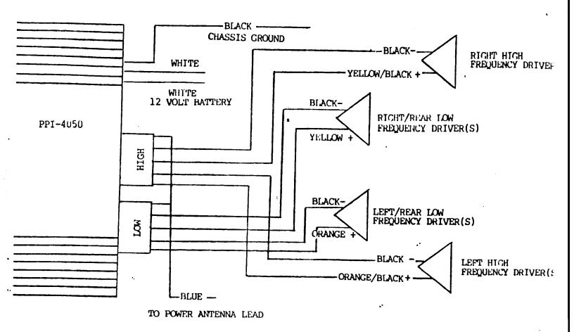
BI-AMPLIFIED SYSTEM/MONO LOW PASS (BOTH SWITCHES IN)
