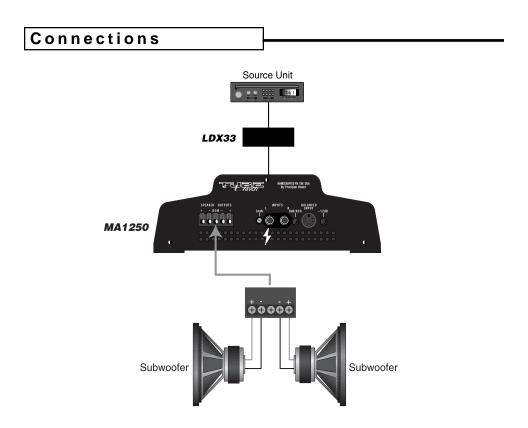
(Two four ohm subwoofers connected in parallel = two ohm load on the amplifier.)
