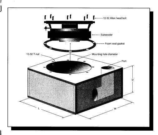
Internal dimensions should be calculated to determine the correct enclosure volume. Be sure to allow for speaker displacement, extra bracing (if used), and port displacement (only the length of the port that is INSIDE the enclosure). It may be necessary to angle the port to fit your design. To calculate the displacement of the port:
