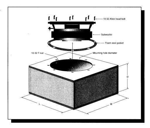
Internal dimensions should be calculated to determine the correct box volume. Be sure to allow for speaker displacement and extra bracing (if used).
