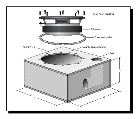
Internal dimensions should be calculated to determine the correct box volume. Be sure to allow for speaker displacement, extra bracing (if used), and port displacement. It may be necessary to angle the port to fit your design. To calculate volume of the port: Radius<sup>2</sup> x 3.14 x Length of port.
